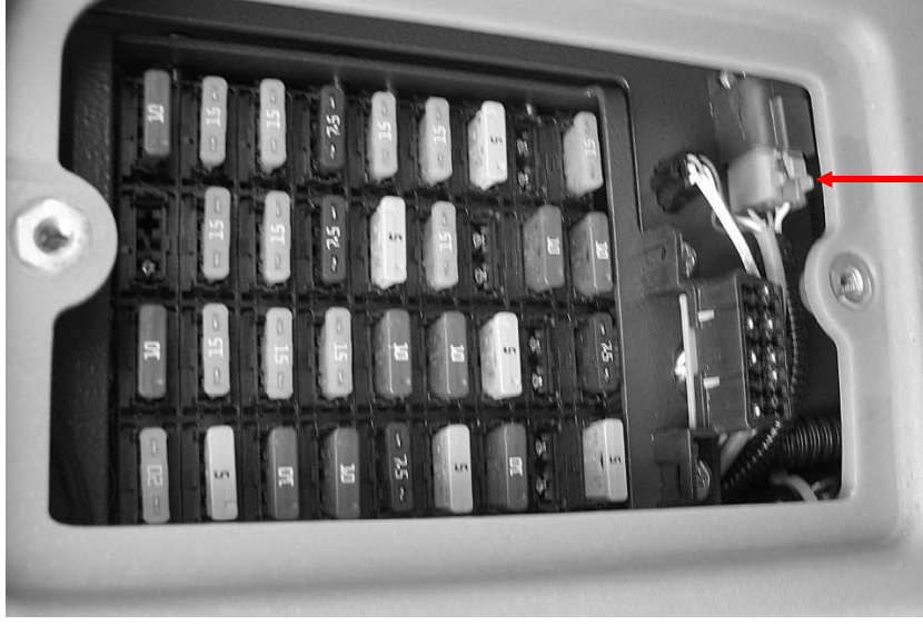
X59 Steckdose 6pol. Diagnose Yanmar X59 Diagnosis Yanmar, socket (plug) 6 pole
